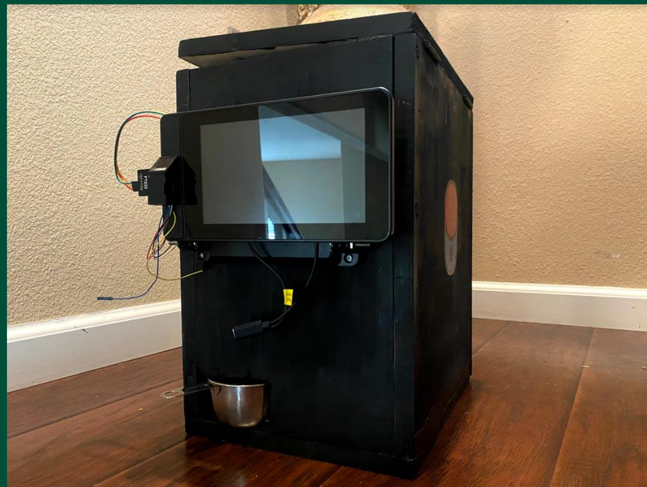
Figure 1. This is the deployable prototype of our pill dispensing device. The touchscreen display is seen at the top, with the fingerprint scanner attached to the left of it, and the dispensing station on the bottom left where the pills come out. Our brand logo can be seen on the left and right panels of the device.
